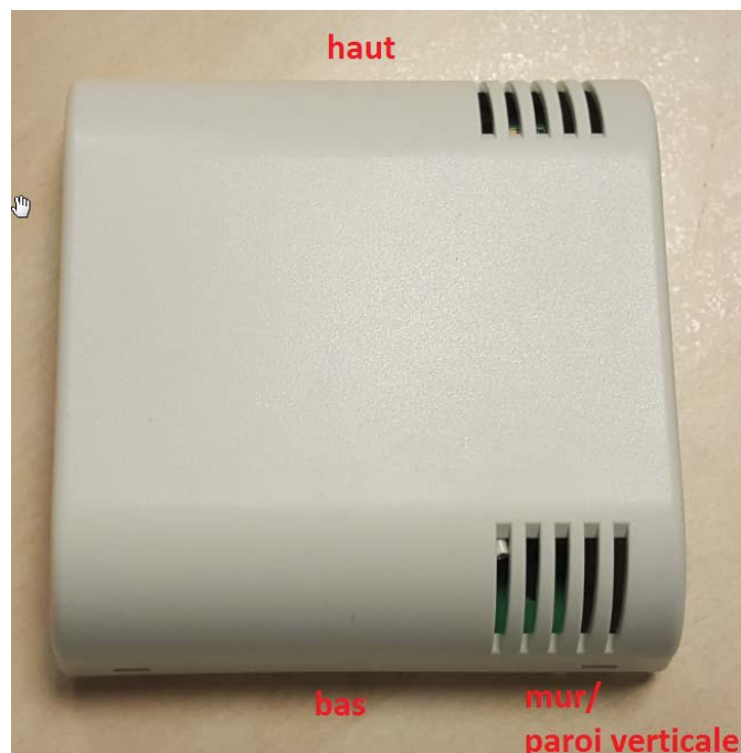
Picture 1 - Sensor mounted on a vertical wall
