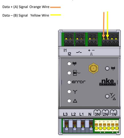
**The RS485 output is activated only the first 5 minutes.** It is possible to activated by pressing the configuraion button on Triphas'O:
