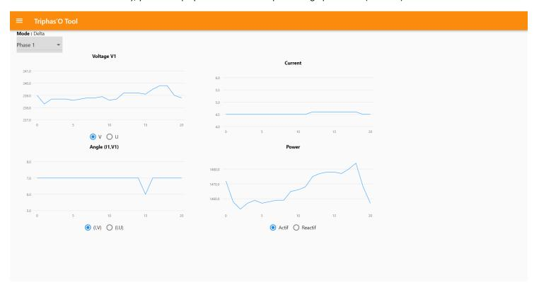
For the voltage and angle values you can select either  $\mbox{\it V}$  or  $\mbox{\it U}$  only for the Delta mode.
